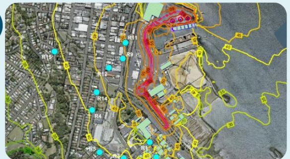
Example of noise modelling from the Port of Burnie over the urban and marine areas
